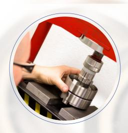
The bearings are completely dismantled; the components are cleaned & measured. In every case the naked bearings are replaced & the rest of the components such as damping springs & bearing bushes are carefully inspected for reuse, in other case they are replaced.
