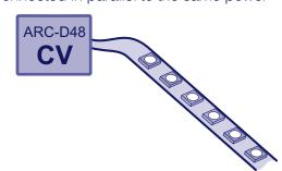
emitters connected in parallel. In such cases, if you tried to use a CC driver, its voltage alterations would produce uneven effects across the multiple emitters, causing imprecise dimming and possibly even permanent damage. In these situations an ARC-D48 CV (constant voltage) driver, with its variable current operation, proves to be an excellent solution.
