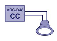
One-Cell fixtures all need a CC driver and our Pro Multi-Cell fixtures have the equivalent CC driver built directly into them.
